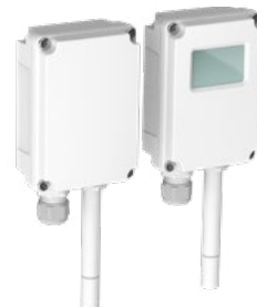
TMW110 Temperature Transmitter, Wall-mounted Accuracy \pm 0.2^\circ\text{C} ( \pm 0.36^\circ\text{F} ) Outputs: 4-20 mA, Modbus RTU IP65 enclosure, optional display Durable design, minimized maintenance needs
