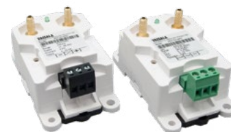
PDT101 Differential Pressure Transmitter Accuracy: 0.4 % / 1 % of span Outputs: 4-20 mA, 0-5 V, 0-10 V Unidirectional/bidirectional options Optional pressure ranges Easy mounting
