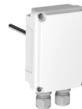
TMI110 Immersion Temperature Transmitter Accuracy \pm 0.1^\circ\text{C} ( \pm 0.18^\circ\text{F} ) Outputs: 4-20 mA, Modbus RTU Installed in a thermowell Precise measurement of liquids Very fast response time
