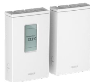
TMW90 Room Temperature Transmitter Accuracy \pm 0.2^\circ\text{C} ( \pm 0.36^\circ\text{F} ) Outputs: 4-20 mA, 0-10 V Exchangeable measurement modules Display with sliding cover
