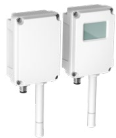
HMW110 Humidity and Temperature Transmitter, Wall-mounted Accuracy \pm 2\% RH, \pm 0.2^\circ\text{C} ( \pm 0.36^\circ\text{F} ) Outputs: 4-20 mA, Modbus RTU IP65 enclosure, optional display Durable design, minimized maintenance needs
