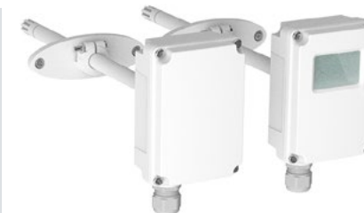
HMD110 Duct Humidity and Temperature Transmitter Accuracy \pm 2\% RH, \pm 0.2^\circ\text{C} ( \pm 0.36^\circ\text{F} ) Outputs: 4-20 mA, Modbus RTU IP65 enclosure, optional display Durable design, easy to install
