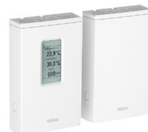
GMW90R Carbon Dioxide, Humidity and Temperature Transmitters Accuracy \pm 1.7\% Rh, \pm 0.2^\circ\text{C} ( \pm 0.36^\circ\text{F} ) Outputs: 4-20 mA, 0-10 V, Modbus RTU Exchangeable measurement modules Display with sliding cover
